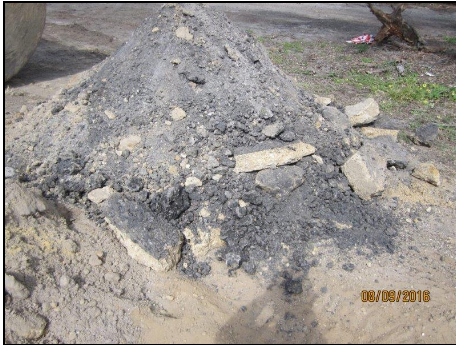
Photo 11: Photograph of black coal washery reject subbase stockpile.
