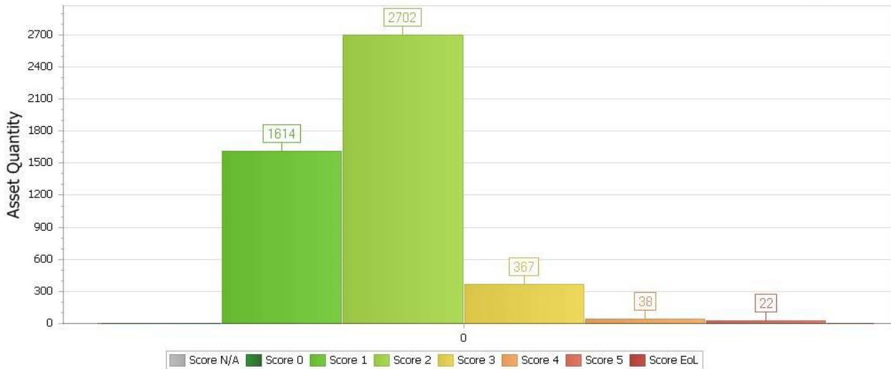
Fig.3.1 Stormwater Pits Assets Condition Rating
