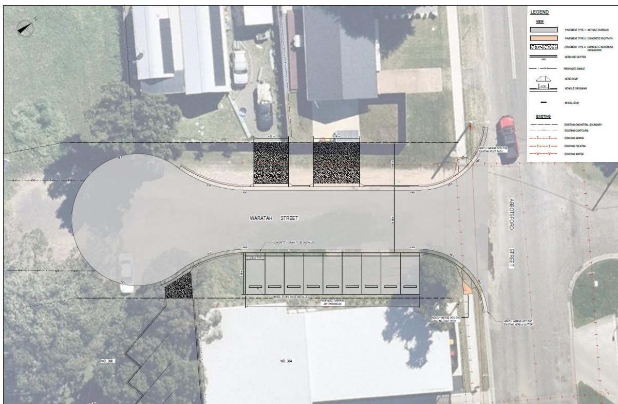
Figure 5: Concept roadworks and drainage plan – Waratah Street
