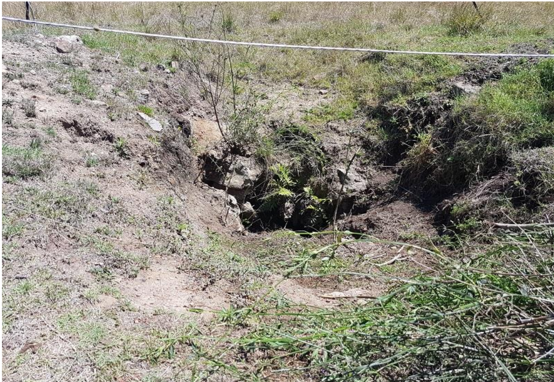
Photograph 9 - Example of pothole from mine subsidence in northwestern portion of the site.
