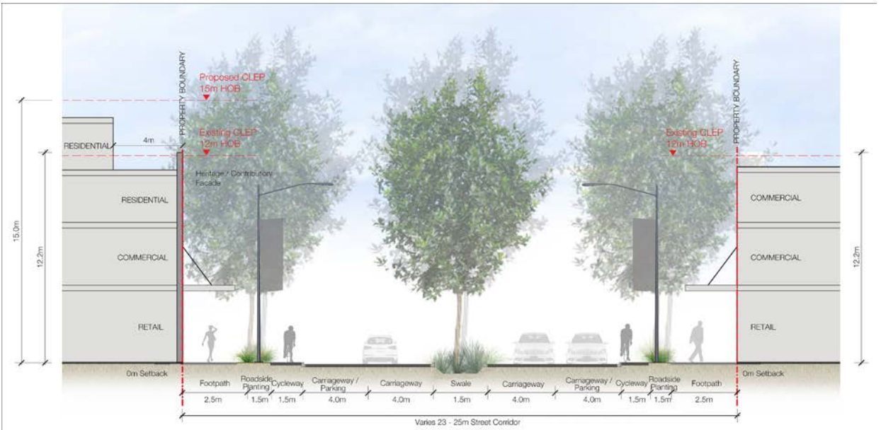
Figure 7: City Bypass/Arterial Road Typology
